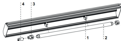
Fig.10 Changing the fluorescent lamp
